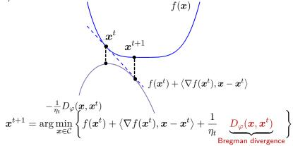
where  $D_{\varphi}(x,z):=\varphi(x)-\varphi(z)-\langle \nabla \varphi(z),x-z\rangle$  for convex and differentiable  $\varphi$
