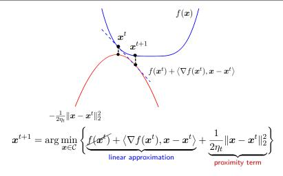
• the quadratic proximal term is used by GD to monitor the discrepancy between  $f(\cdot)$  and its first-order approximation
